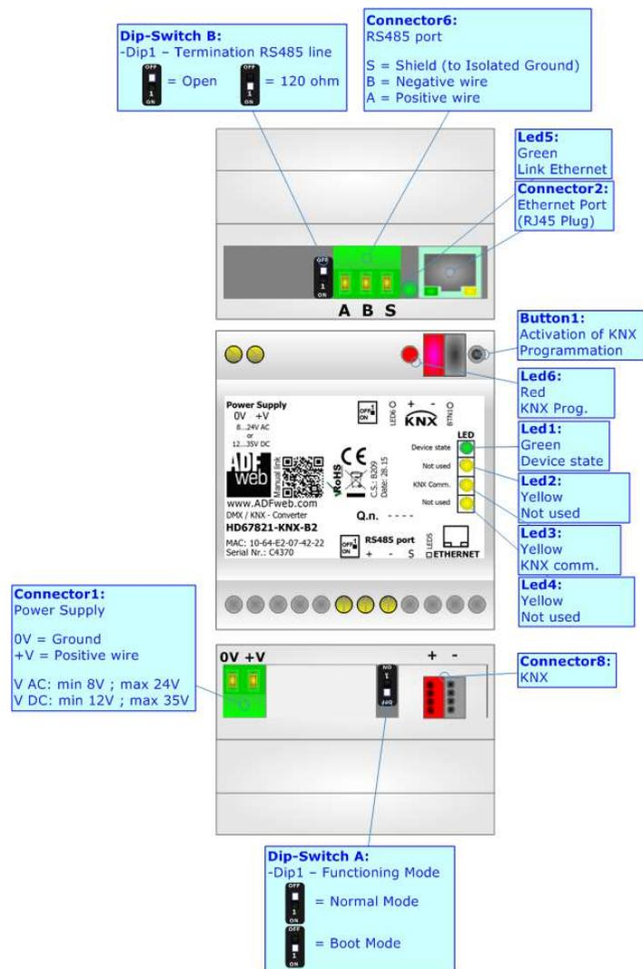
Figure 1: Connection scheme for HD67821-KNX-B2
