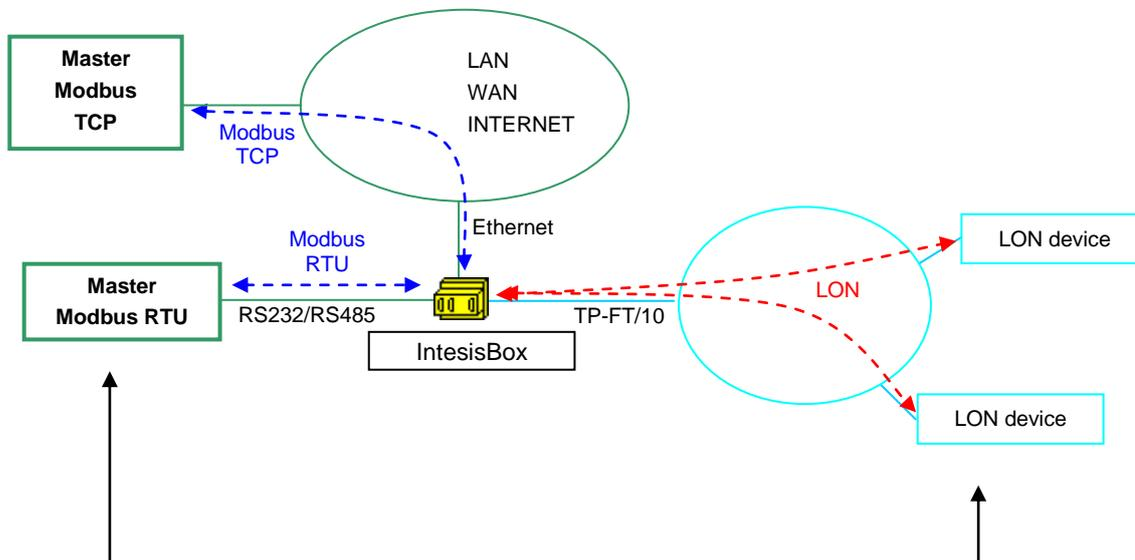
**Control system with Modbus master interface:**
